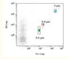
MP gate set-up 0.5 to 1 µm standard MP gate
